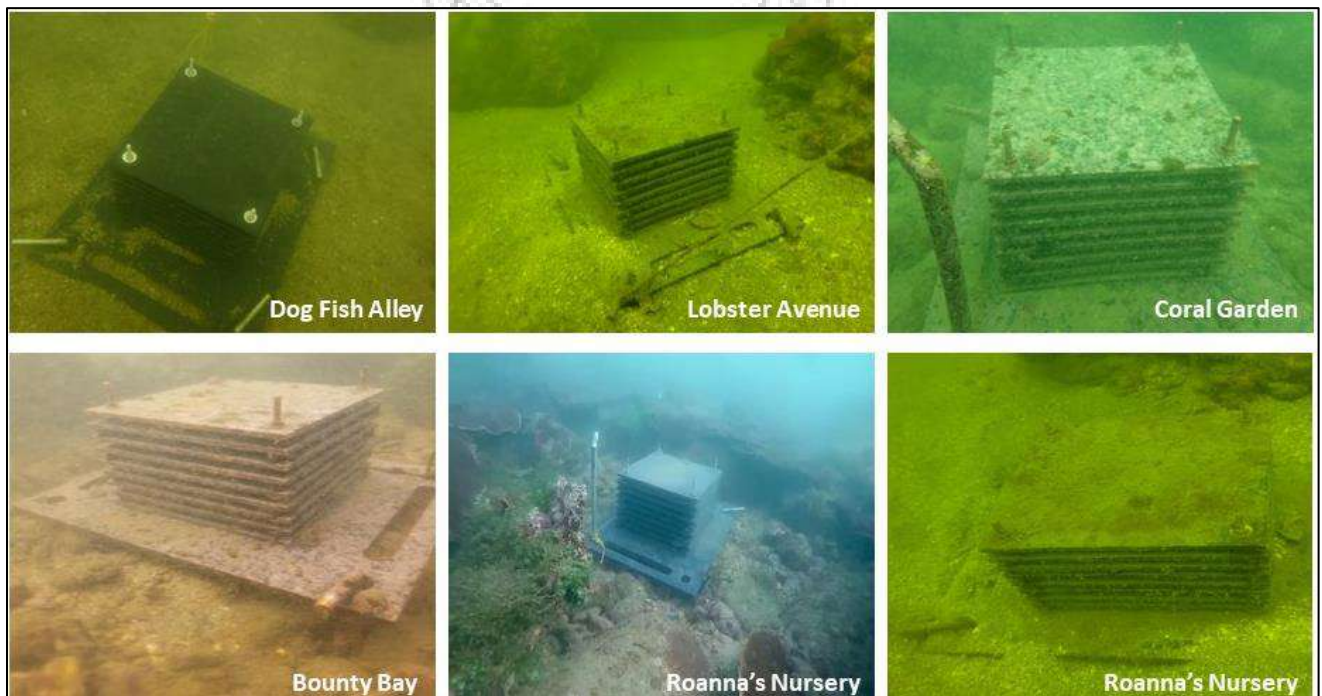
Figure 6: Images of the ARMS deployed in the Grande island coral reef environment
